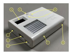
The ConnectBox is a self contained WiFi hotspot allowing the user to distribute pre-loaded media content simultaneously to up to 17 users. It is battery powered with a run time between charges typically 6 to 8 hours. The following are simplified instructions for its use. More detailed information can be found in the **full document** at:
